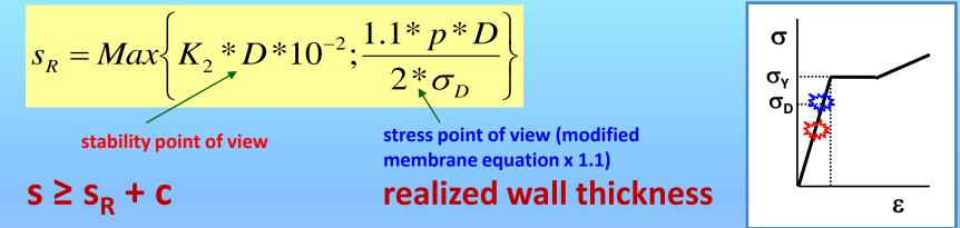
Coefficient K<sub>2</sub> is determined from diagram in the standard (more in the part 8 "Stability of beam plate and cylinder")
