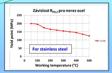
where is:pcalculated (working) pressure $\sigma_D$ allowable stress at calculated temperature $\sigma_{D20}$ allowable stress at temperature 20 °C (pressure test<br/>temperature) $x_{WP} = 1.5$ safety coefficient for working pressure $x_{PT} = 1.5 / 1.35 = 1.1$ safety coefficient for pressure test  $\rightarrow \sigma_{PT} = \sigma_Y / 1.1$
