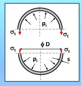
In tangential direction  $F_{et} = F_{it} \rightarrow$   $p_i * D_i * L \approx 2 * L * s * \sigma_t$   $\sigma_t = p_i * D_i / 2s = p_i * r_i / s$  $s = p_i * D_i / 2^* \sigma_D = p_i * r_i / \sigma_D$
