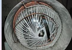
**Cryogenic vessels for LN2 storage (-196 °C)** The vessel has 2 shells and inside is vacuum + thermal insulation wound on the internal shell (layers from special paper + shiny Al foil)  $\rightarrow <<<$  heat loss due to convection, conduction and radiation
